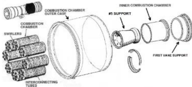
Conducted: Weld repaired the damage on the combustion chambers. Grit blasted to clean the remaining six combustion chambers. Grit blasted to clean combustion chamber clamps. #5 support was cleaned, and pressure tested.
